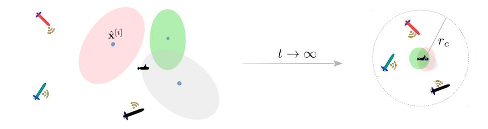
"Optimal" vehicles-target relative geometry for target localization purposes [from the MPC approach]
