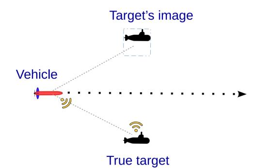
Can not distinguish "True target" and Target's image when using range measurements (because the distances to the vehicle are equal)
